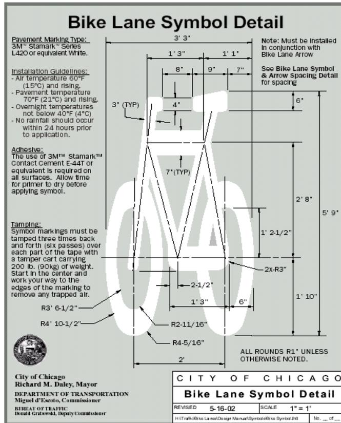
Figure J-1: Sample Design Standard for Pavement Markings
